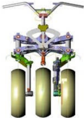
CYCLE PARTS The innovative parallelgram suspension, an original Piaggio design, is anchored to the frame. The tilt mechanism is composed of four cast-aluminium control arms with four hinges fixed to the central tube and two guide tubes on either side of the parallelgram, connected to the arms via suspension pins and ball bearings. The tubes on the right and left enclose the steering tube in a classic singlearm setup.
