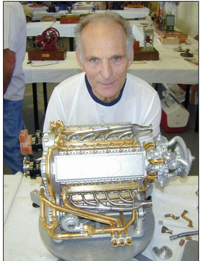
Last month we ran a blurb on a slick, fully functional (well, almost) paper V-8 motor. This month here's what may be the most detailed **computer (CNC) generated V-12 model engine**. The builder is Clennel "Clen" Tomlinson, a 71-year old retired electro/mechanical engineer, living in West Sussex England. This guy's resume reads like a dream with regards to his automotive background. Check this, and other incredible one-offs, at <http://www.craftsmanshipmuseum.com/>.
