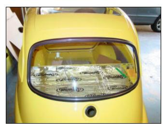
Dynamat Extreme acoustic and heat insulation on rear deck of Bruce's car. New window seal, lock strip and external rubber seals have just been installed too.
