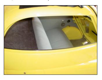
Brand new seat, side panels and carpet in Bruce's car. Door panel is next. The door panel was easily the biggest time consumer in terms of labor to reconstruct a new one even though the original was used for a template.
