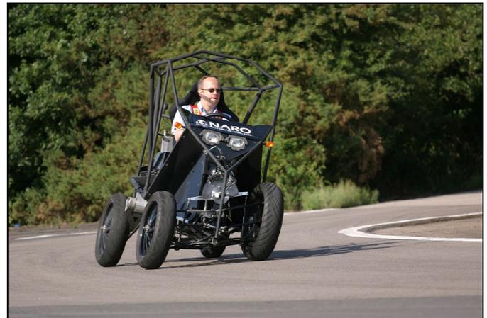
or without, this is one neat ride! **Scott Isensee** sent us the above pix and article on the **NARO** concept vehicle. It's designed for city use as a personal commuter, a taxi or a delivery vehicle, is intended to return over **100 miles per gallon** from a 400 cc, single-cylinder, 4-valve gasoline engine with a maximum of 20 HP.
