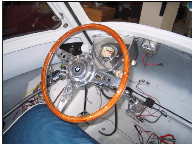
Richard Lewis keeps a steady stream of Rally Isetta updates coming our way. Looks like the **French LeCarra wheel** has found its way onto the steering column where it belongs. This picture doesn't do the extensive polishing job justice but it would appear that Mr. Lewis has gone through a 55 drum of jeweler's rouge in the process of tweaking all that aluminum. By the way, all of Richard's resto pix can now be found at [www.rallyisetta.com](http://www.rallyisetta.com).
