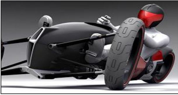
Don't have enough toys? How about this prototype magnetic tricycle? It's about time the dudes cranking this neat stuff out get it on the market. This bad boy uses a 550cc motorcycle engine supplemented by an electromagnetic motor at each of the three, hubless wheels. A French motorcycle manufacturer produced this rendering based on a Finnish design student's composite which was inspired by the combination of a motorcycle and Formula One car.
