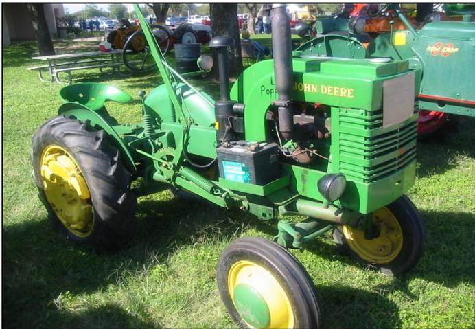
What the @#!\*%&@ has this tractor got to do with microcars? Well, it has four wheels (although some look like they only have three from certain angles), an internal combustion engine, a steering wheel, it's goofy looking and (drum roll) **it's the smallest John Deere tractor ever built**. Micronut's roving reporter **Robert Mace** advises *ALCN* that it's a **1944 Model LA**, that cranks out 13.1 horsepower, .4 HP less than an Isetta. Bubba's
