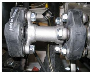
On the right, we've got some genuine BMW guibos (drive donuts for the rest of us) to beef up the drivetrain. Below right are the cool rally lights. On the left is a shot of a custom-machined tow/tie-down hook mounted on the chain drive. Neat!
