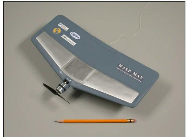
The **WASP MAV** (Micro Aerial Vehicle) is hardly a car but it IS a micro. This deal is being developed for military surveillance. The seven-ouncer is currently being tested by the **Nimitz Carrier Strike Group**. We need one of these, too.
