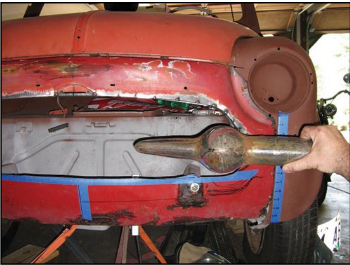
Front bumperettes made from components of 1956 Buick front bumper and 1951 Mercury accessory grille guards.
