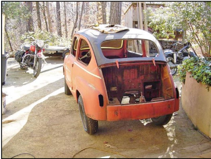
December, 2004: Lower body reinforcement done, the car heads into surgery for the "topectomy".
