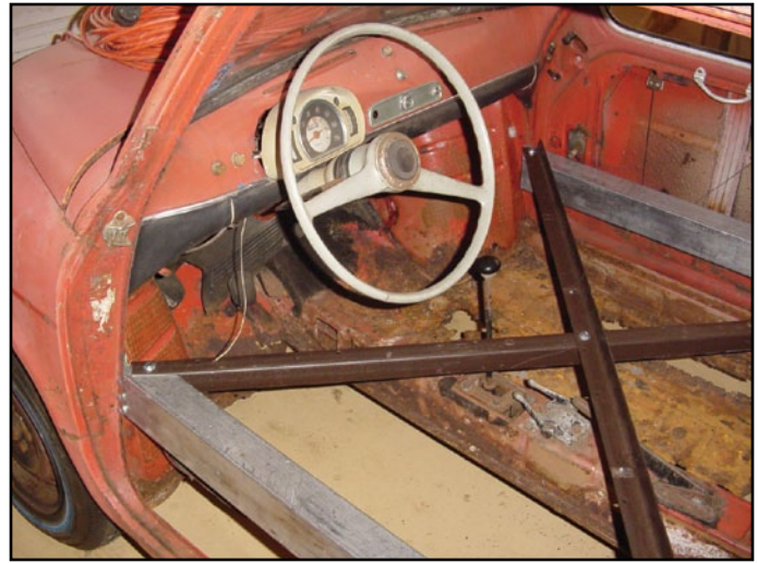
Once the car is home, I started bracing the body to maintain its continuity while all the rusty metal is being tended to.
