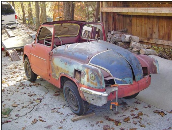
Begin the reconstructive work. Deck lid was a 1953 Chevrolet truck hood, quarter panels were from a 1953 Pontiac and rear bumper section from a 1956 Buick.
