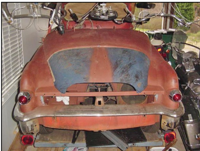
Begin the reconstructive work. Deck lid was a 1953 Chevrolet truck hood, quarter panels were from a 1953 Pontiac and rear bumper section from a 1956 Buick.
